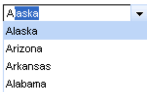
Figure 6.20. <rich:comboBox> with "directInputSuggestions" attribute.
